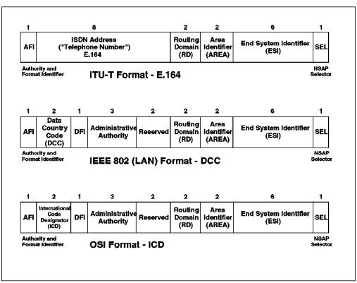
Figure 1. ATM Addressing Format Cell
